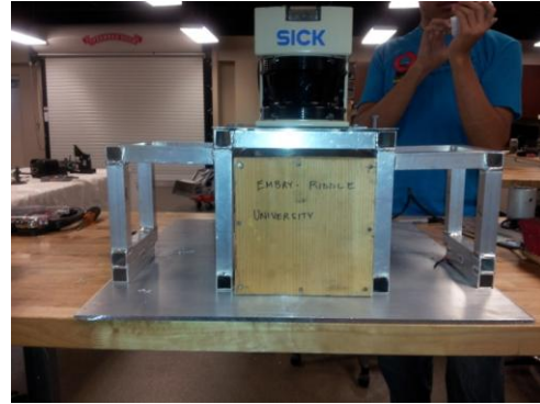
Figure 3 Payload cage in the middle with battery cage on either side. LRF on top of steel plate.
